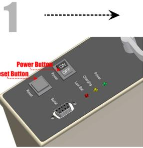
1 Connect all sensors to DCU. After powering on the DCU, press the reset button.
