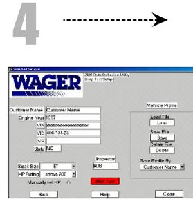
4 Fill in fields for customer test set up. Then Press "Start Test" Button.
