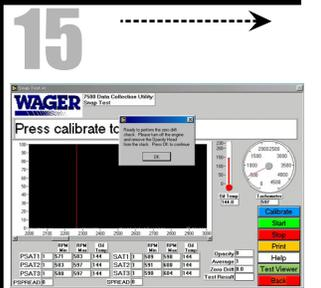
15 Perform the "zero drift check" by pressing "OK".
